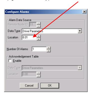
Once we have setup the ALARM register, we can now create the ALARM or Fault Screen itself.
