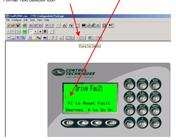
Parameter #10.20 in the Unidrive will indicate the Fault Code of the last trip. We would want to decode that into a text phrase.
