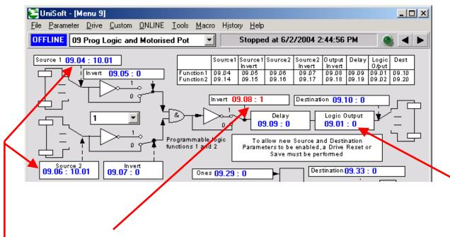
We would set the Gate inputs to monitor the Drive Healthy bit (#10.01) and invert it by setting #9.08=1.
