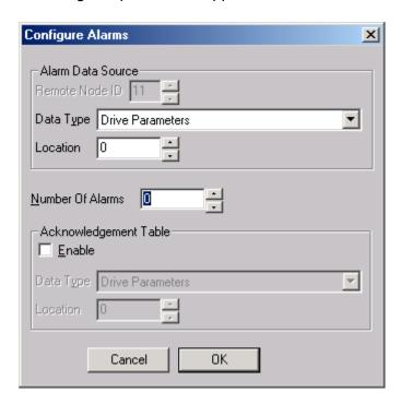
The configurator is looking for a location in the drive that becomes a 1 when an Alarm is to be displayed. Unfortunately, the Unidrive creates a 1 when the Drive is Healthy at parameter #10.01. We need the opposite.
